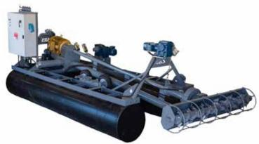
A floating lagoon structure solves an industrial and municipal environmental issue by removing settled waste and other by-products from ponds or lagoons.
